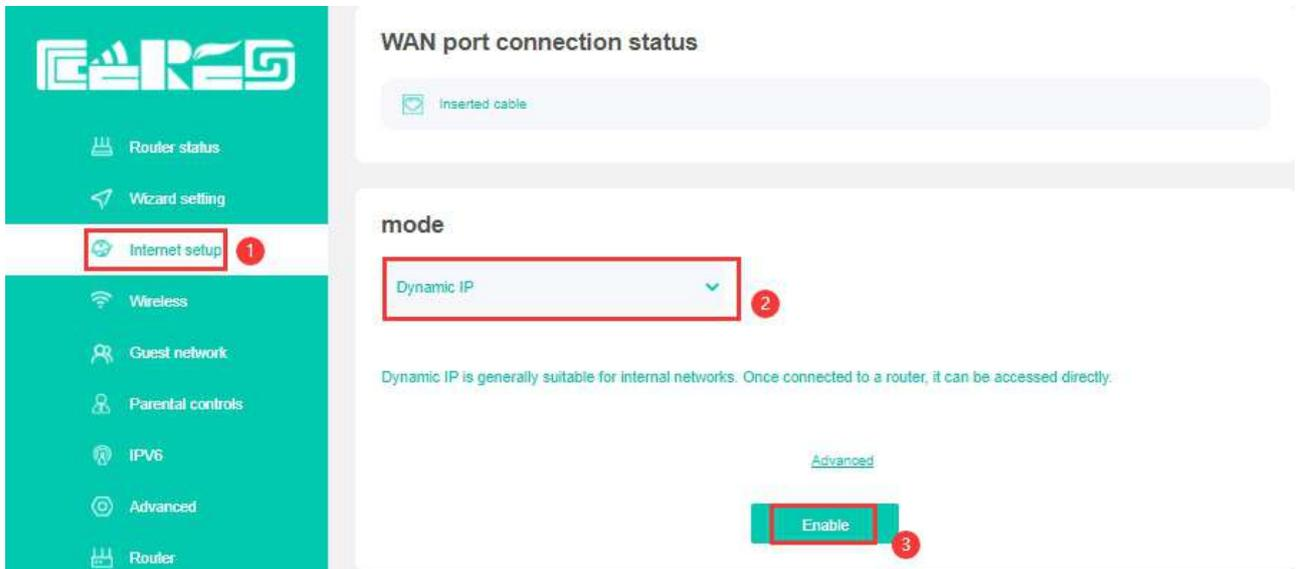
After finished all of the configuration,click **‘Enable’** button to finish **“DHCP”** setting.
