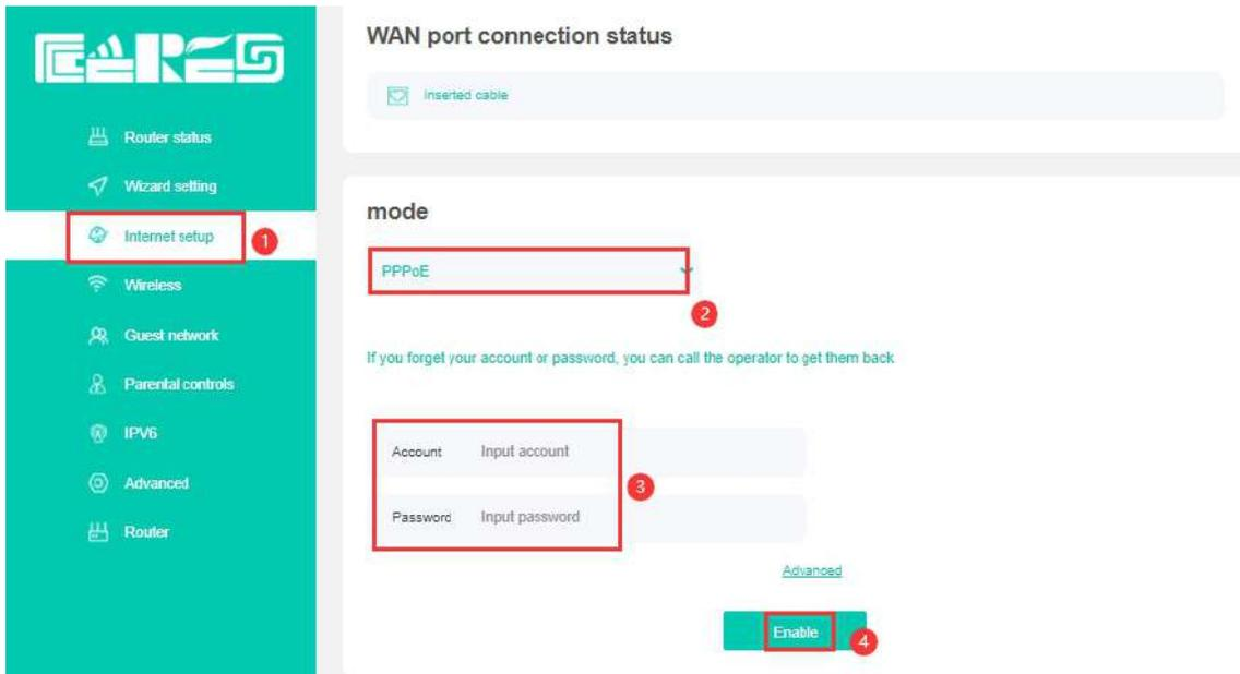
After finished all of the configuration,click **‘Enable’** button to finish **“PPPOE”** setting.
