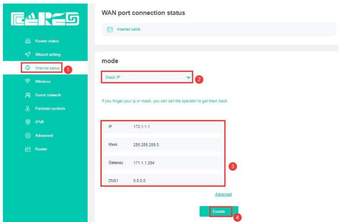
After finished all of the configuration,click ‘Enable’ button to finish “Static IP” setting.
